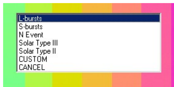
Illustration 41: The customizable Annotate pop-up menu is accessed by right clicking on a loaded spectrogram and selecting Annotate or Annotate Region.
