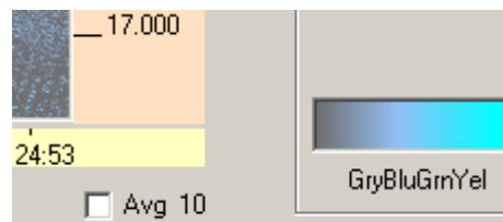
Illustration 18: Checking the "Avg" box forces the averaged view of spectra. The number of spectra averaged is set under the Spectrogram menu.
