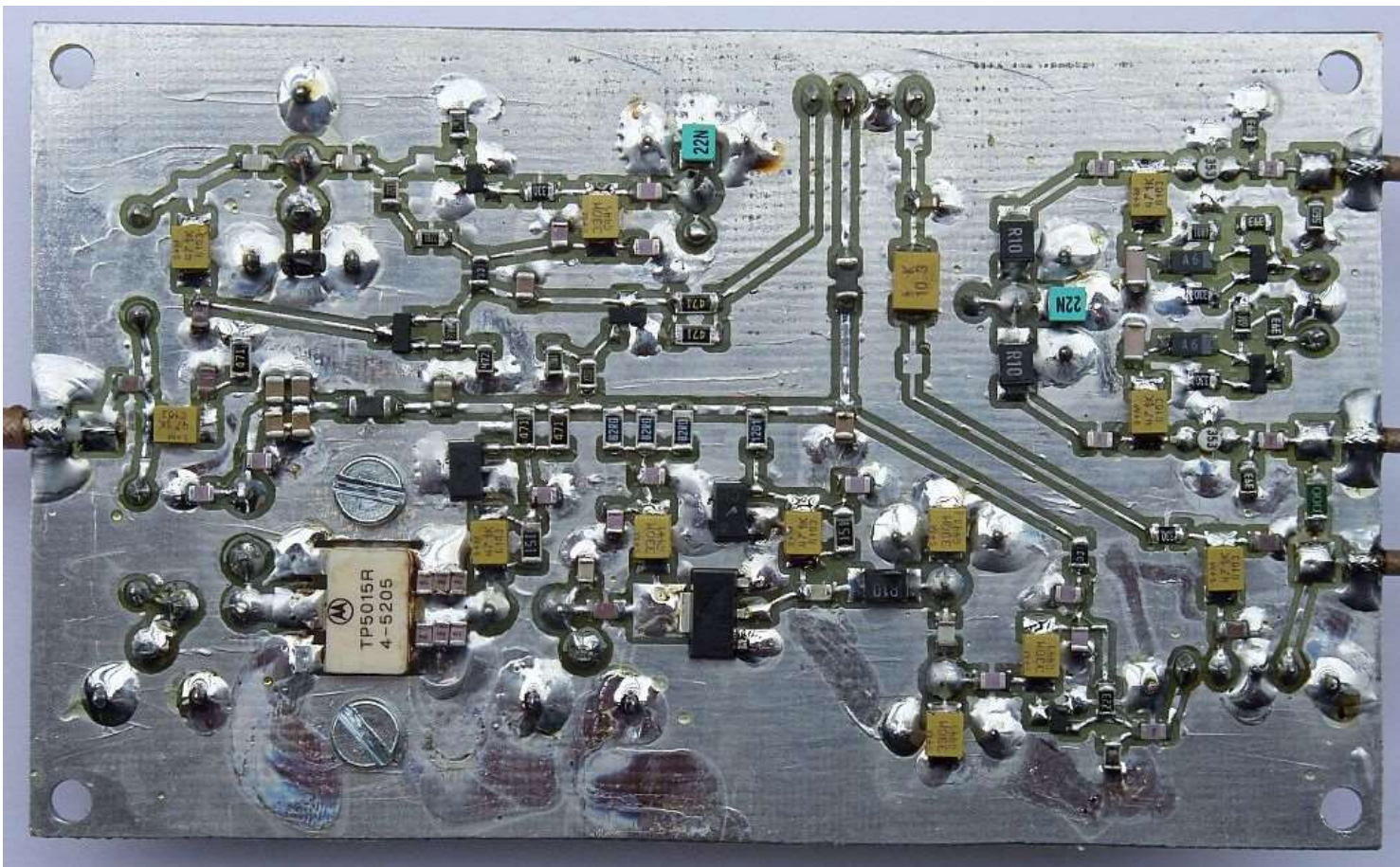
The ZIF chain includes an AGC stage (74HC4066), two NE592 amplifiers (SOIC-8 version) and a Costas-loop demodulator programmed into an Altera EPM3032ATC44 CPLD. The inputs of the latter are biased into linear operation to accept analog signals directly without additional comparators. The Costas loop uses a DPLL/1024 in the version for 1.2288Mbps, 430MHz:
